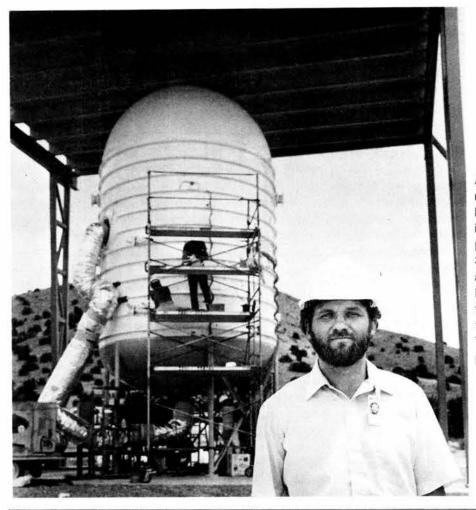
A MODEL of a steel nuclear reactor containment building (1/8th scale) is being instrumented for high pressure tests scheduled in September to validate analytical codes used by NRC to predict behavior of the structures in an extreme accident scenario. Tom Blejwas (6442) is the project leader.
